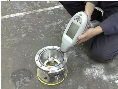
Figure 2 PMI Testing of Component using Hand Held Meter
